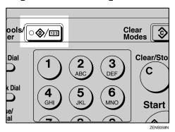
Press the ② or ⑤ key to display "5.Printer Features", and then press **[OK]**. The following screen appears on the panel display.
